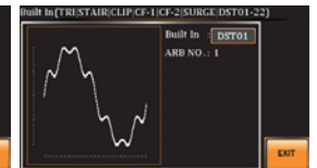
Fourier Series Synthesized Waveform
