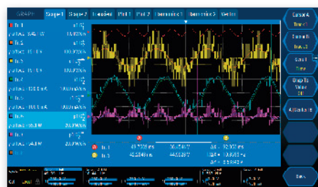
Simultaneous measurement of narrowband and wideband values
