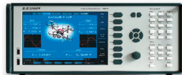
LMG triggers on data or commands from CAN bus and executes actions (e.g. starts a log)
